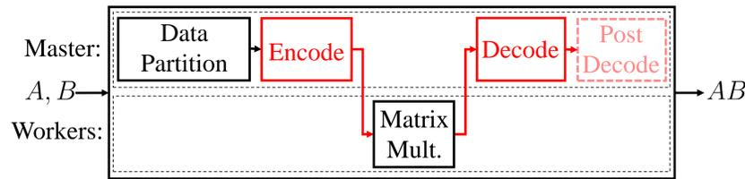
• **Encoding** via polynomial basis :  $\{T_k(x)\}_{k=1:K}$ ,  $K = 2$ .
